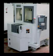
After in-house preparation of the billets (cutting, deburring, marking etc.) the secondary operation is carried out on numerically controlled lathes with robot loader or on the machining centre equipped with a roto-pallet system and NC rotary tables.
