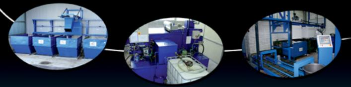
Ground pollution is avoided by storing under shelter waste and lubricants, both new and used, in barrels, sealed containers or "3D PACK" type reservoirs. Oil mist is controlled by having special air extractors on each machine so that there is no pollution of the outside air.
